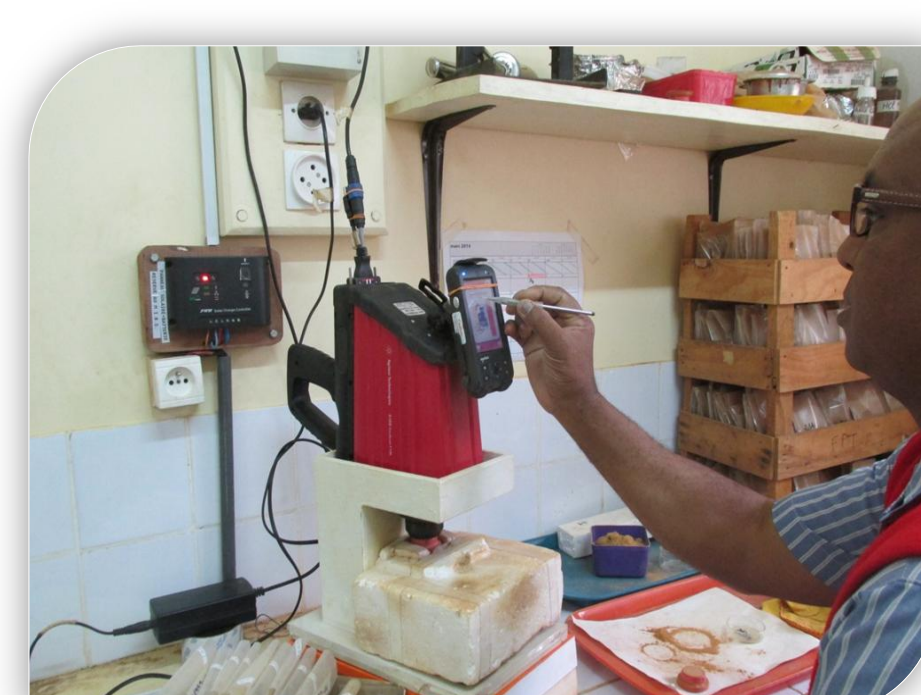
Photo 3: Spectrometric analysis to determine carbon content
