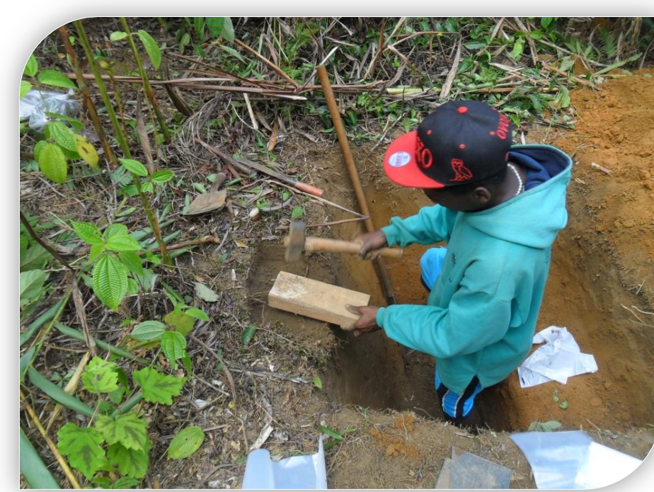
Photo 2: Soil sampling by cylinder for bulk density
